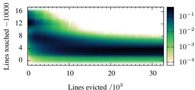
Figure 6: Exynos4412 cache channel with IBS.  $N = 1000$ ,  $B = 400$  b/s,  $CI_0^{\max} = 1.2$  b/s.
