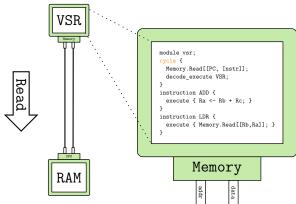
The cycle specifies asynchronous behaviour.
